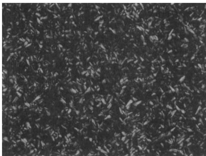
Figure 1. Optical micrograph showing the characteristic batonnette texture of a lamellar phase for the APFO/EG system ( w=0.65 ) at 213 K (magnification 200x).
